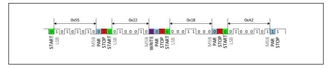
Figure 22: Example of Read (Reg[0x2B], Reg[0x2C])
