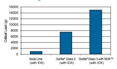
It takes more load to initiate radial cracks in the glass.
