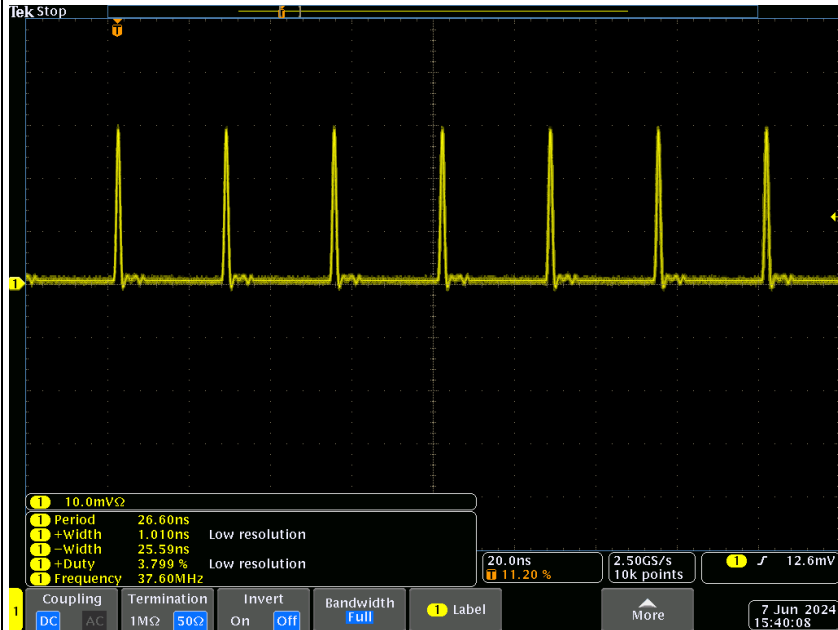
FIGURE 2 – Model TMF8806 – Pulse frequency – 40MHz, Pulse Width setting – 1, Pre pulse setting – 0, PrePulse Width 2x setting – ON, Peak Current setting 15
