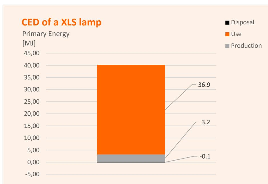
A potential measure to reduce the primary energy consumption of signal lamps in cars is the replacement of the incandescent lamp technology with LED technology. Compared to a traditional signal lamp (P21W – 7506) savings up to 73% can be achieved.
