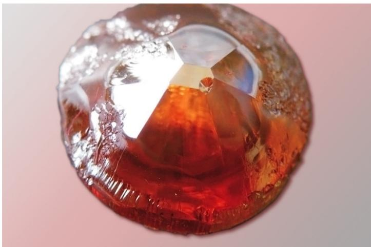
An aluminum nitride crystal which has to be produced as the basis for the UV LED.
