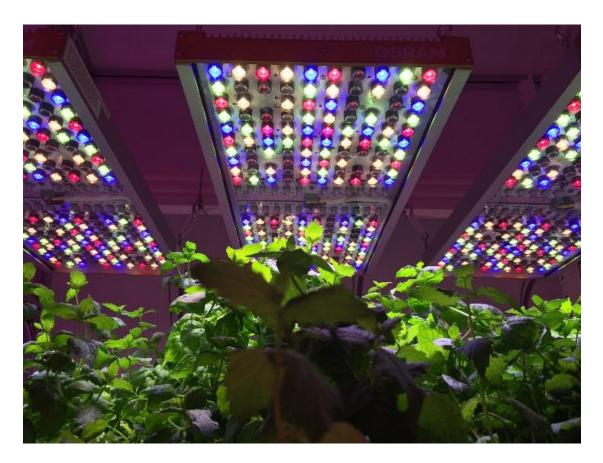
Each of the six spectral channels can be addressed individually with Phytofy RL and the intensity planned and managed precisely in real time.
