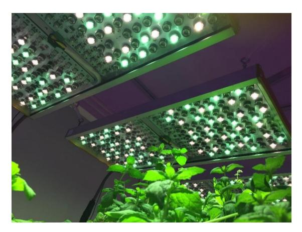
Use of Phytofy RL allows the researchers to evaluate the most varied light recipes, without having to change luminaires between individual tests. Picture: Osram
