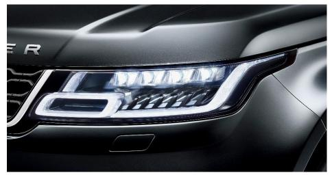
Innovative SMARTRIX modules from Osram provide the basis for the fresh angular design of the headlights on the 2018 Range Rover Sport. Picture: Jaguar Land Rover
