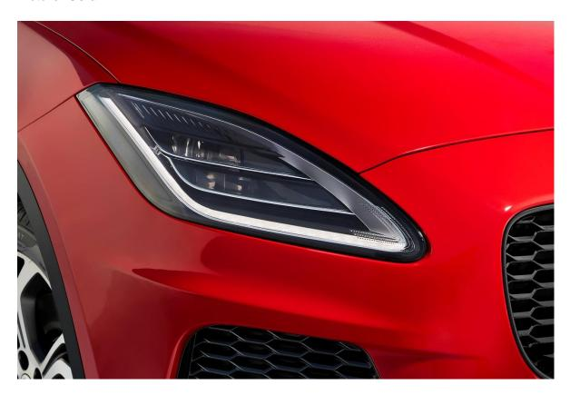
The innovative SMARTRIX modules from Osram contribute to the particularly compact design of the headlights on the new Jaguar E-PACE.
