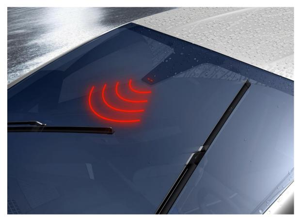
Photodiodes SFH 2200 A01 and SFH 2200 FA A01 are ideal for rain sensors that detect when the windshield wipers need to be activated. Picture: Osram
