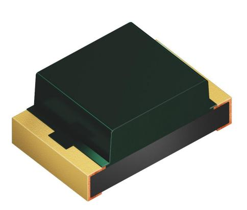
Ambient light sensor SFH 5701 A01 is an active component in which the IC is powered by the signal current and therefore does not need an external power supply. Picture: Osram
