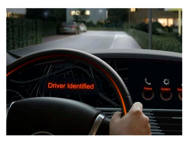
Biometric driver identification thanks to the two IREDs offers numerous benefits, such as automatically unlocking the immobilizer or adjusting the individual seat position. Picture: Osram
