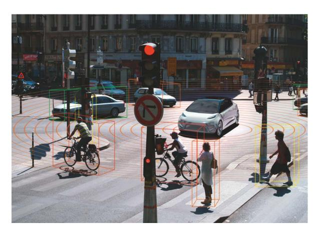
LiDAR systems use the propagation time of laser pulses to calculate the distance between the vehicle and people or objects.
