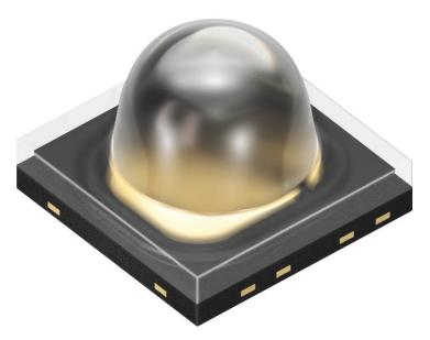
With the new SFH 4718A the Oslon Black family now offers a wide selection for the most varied of infrared-based applications, taking in four power classes, three wavelengths and three beam angles.
