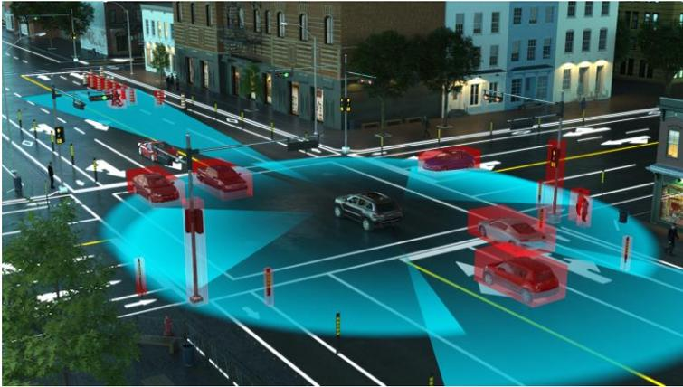
LiDAR (Light Detection And Ranging) is similar to radar technology in that it detects objects and measures distances and speeds, but it is based on infrared light.
