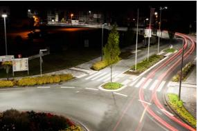
Streetlight 10 Midi luminaires with a special reflector for optimum illumination of pedestrian crossings.
