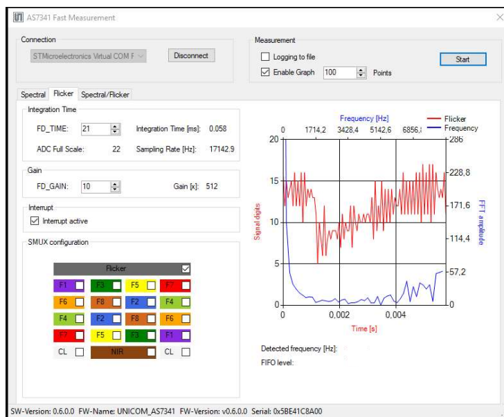
Figure 20: Rushing Results Based on Too Low Integration Time
