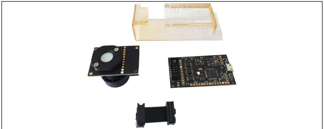
Figure 6: Sensor and Standard Unicom Board Connected via Ribbon Cable, USB-Interface, and an Insertable Plastic Housing
